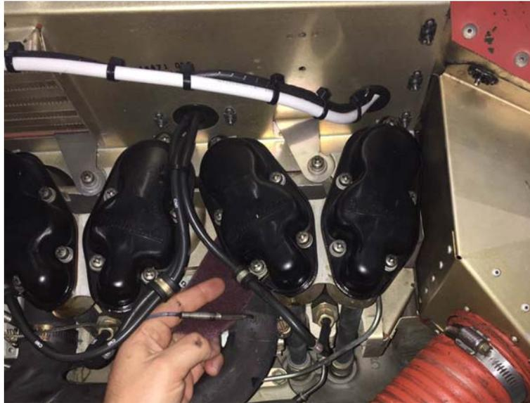
Figure 11. Deburring with Scotch-Brite™ Pad
