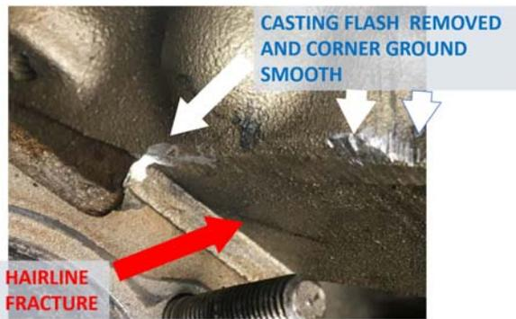
Rework performed on cracked cylinder
