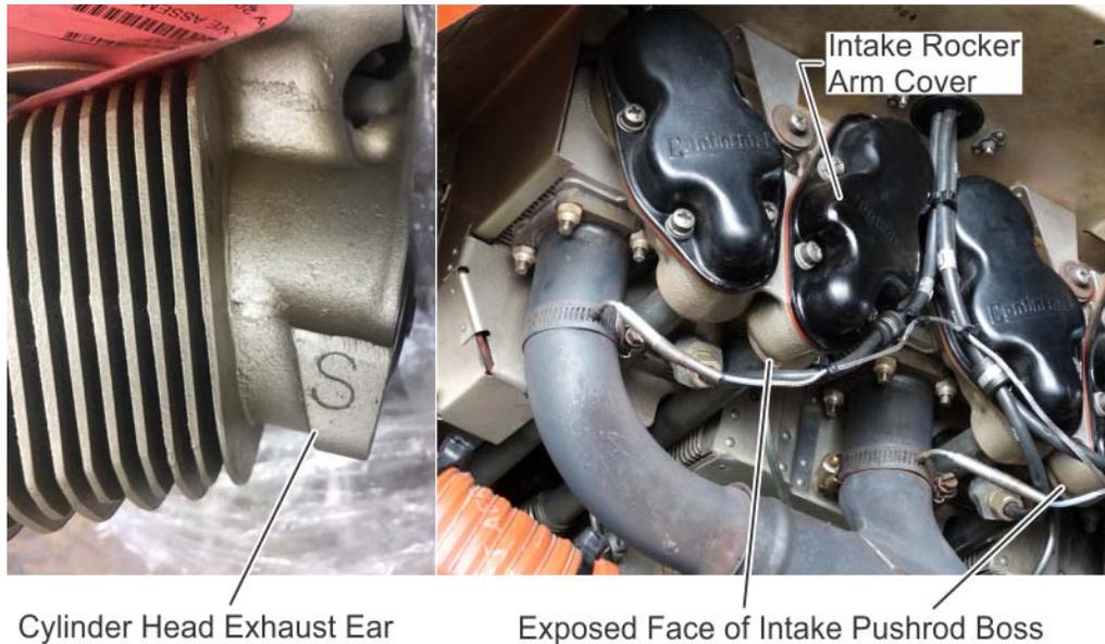
Figure 4. Cylinder Head Indicates Prior Compliance, Stamped with Letter “S”
