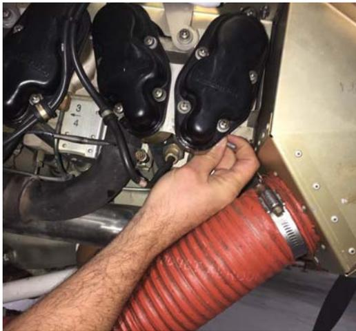
*File inserted behind intake valve ear, working horizontal edge*
