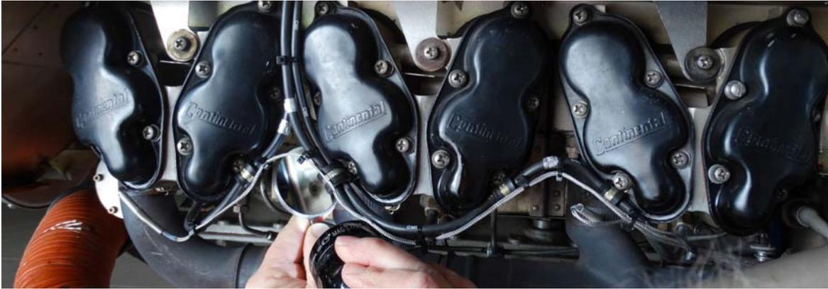
Figure 6. Cylinder Head Inspection Area, typical aircraft installation
