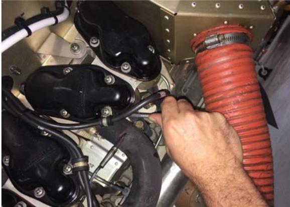
*File inserted behind exhaust valve ear, working vertical edge*
