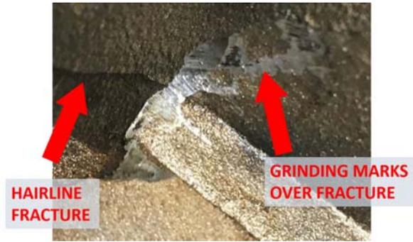
grinding marks through crack - closeup
