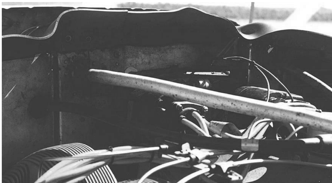
Figure 6-77. Improperly Positioned Aft and Side Peripheral Baffle Seals
