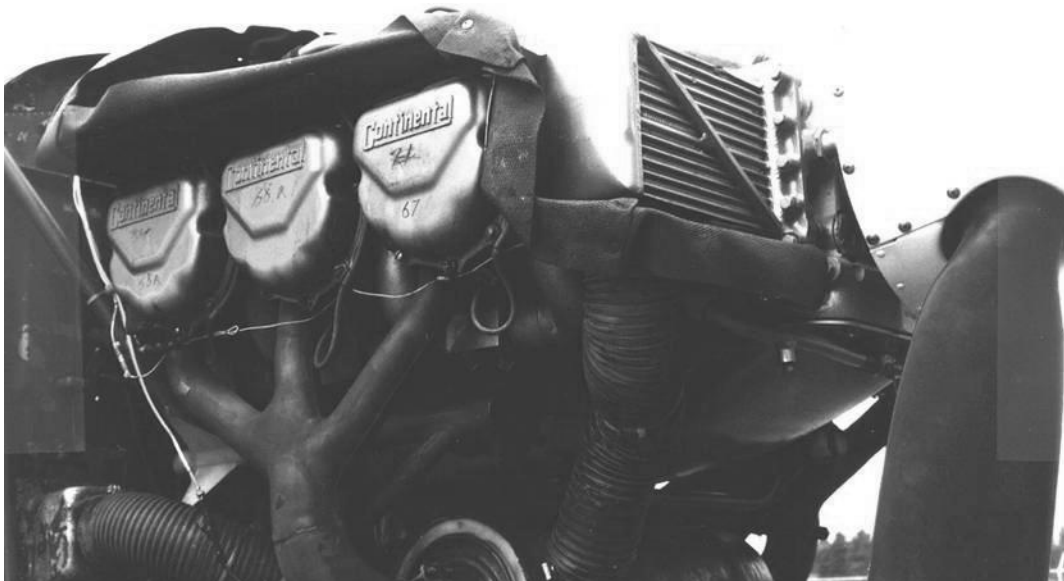
Figure 6-76. Improperly Positioned Baffle Seals
