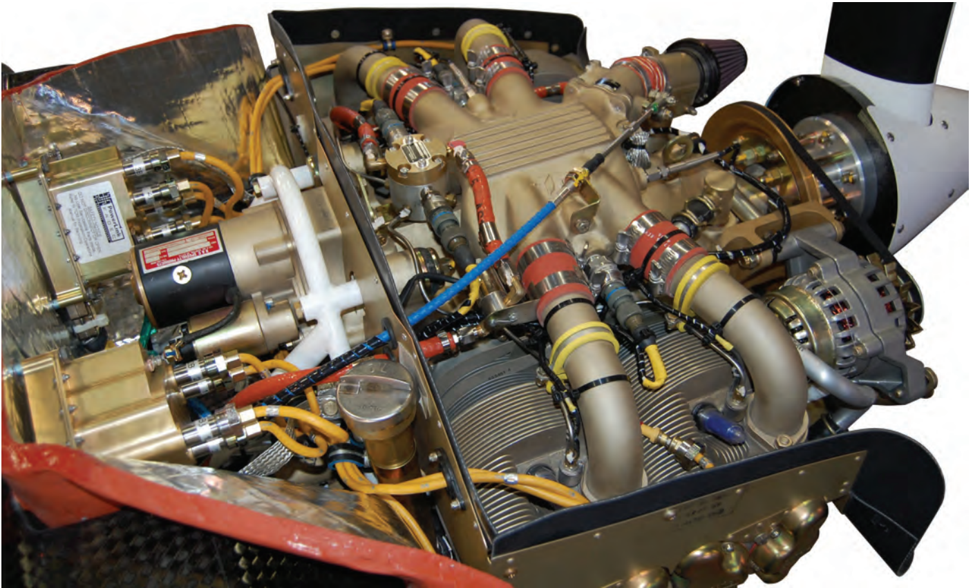
PowerLink FADEC IOF-240-B installed in certified Liberty XL2 Aircraft
