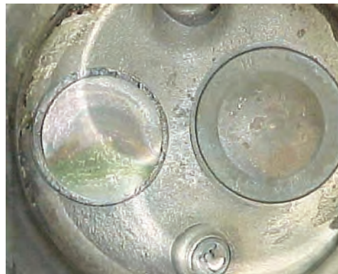
Burned Exhaust Valve
