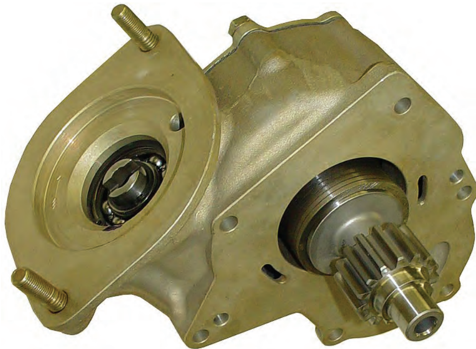
Photo of a Typical Right Angle Starter Adapter used commonly on 470, 520 & 550 "Sandcast" series engines.
